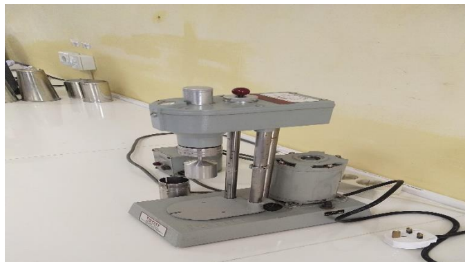
Gambar 3. 3 Fann VG meter (Laboratorium STT MIGAS Balikpapan,2024)
